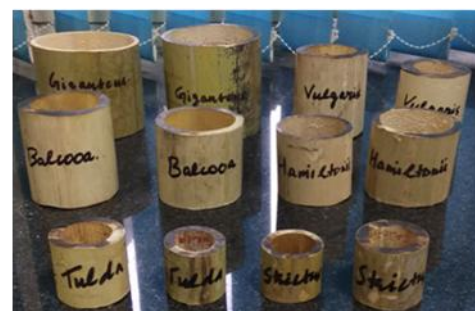
(b) Compression Strength Test Blocks
