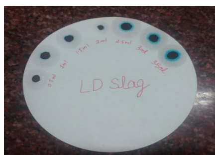
Fig. 4: Methylene Blue Test
