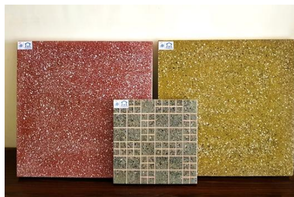
Fig. 3: Developed Mosaic Flooring Tiles using 80-85% Marble Waste, by weight
