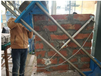
Fig. 5: Test Setup for Diagonal Compression & Shear
