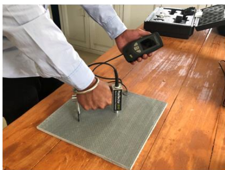
(a) Barcol Hardness Test as per ASTM D2583
