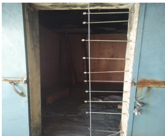
Fig. 1: (c) Bi-Directional Probes at Door Centre
