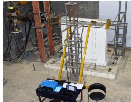
Fig. 2: Lateral Load Test of Precast Wall-Column
