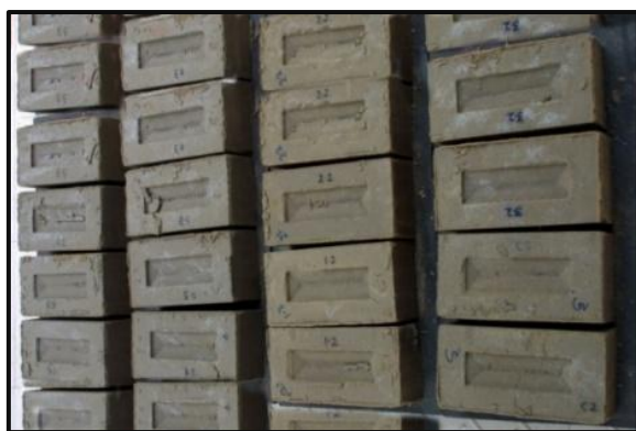
Fig. 1: Bio-Bricks using Desert Sand & Bacteria
