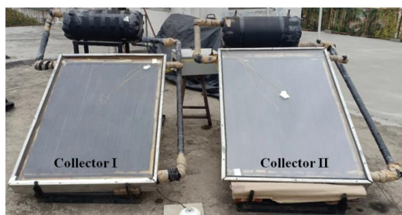
Fig. 1: Two Prototype of Double Glaze Flat Plate Collector
