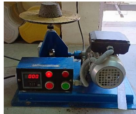
Fig. 16: Flow Table Setup
