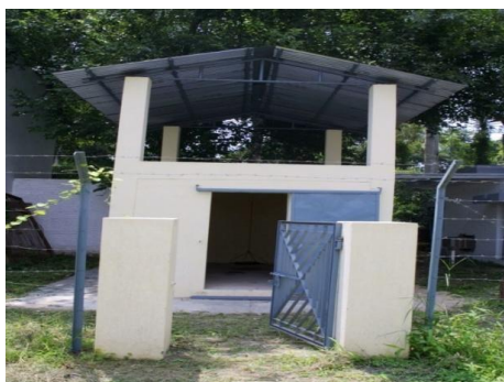
Fig. 1: (a) ISO 9705 Full-Scale Room Corner Fire Facility
