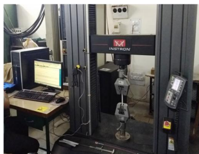
(a) Tensile Test as per ASTM D638
