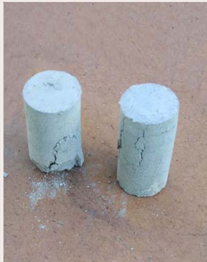
Photo 2: Failure Pattern of Stabilized Sample by UCS Test
