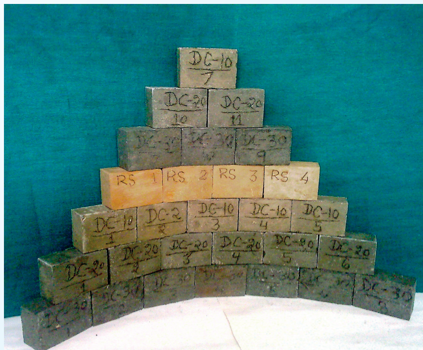
Fig.5 : Experimental briquette samples (7.5x5.0x3.5cm) prepared using Raipur soil & Sponge iron waste
