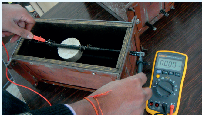
Fig. 3: Attachment of Galvashield XP anode and connectivity checking
