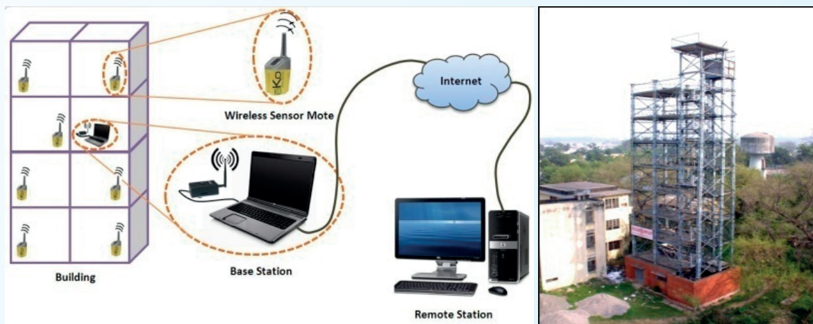
Fig.1: Schematic of structural health monitoring data flow using wireless sensor network
