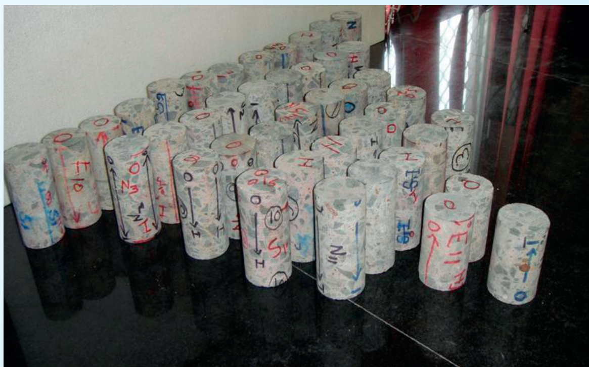
Fig. 2: Concrete core samples extracted from the Cooling Towers
