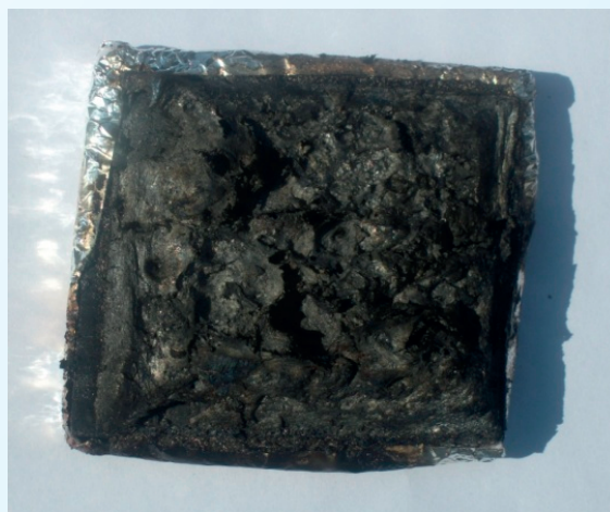
Fig. 3: FR Plywood before & after exposure to Cone Calorimeter
