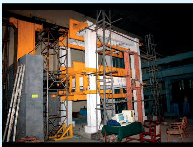
Fig. 1: Test setup for full scale testing of '3-S' Model under quasi-static condition
