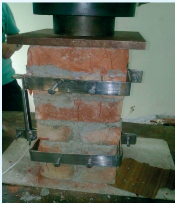
Fig. 1: Testing of Bricks for splitting tensile strength test as per ASTM standards
