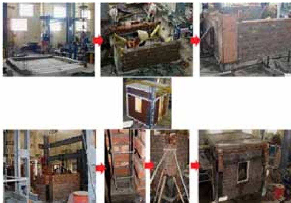
Fig.1: Sequence of construction of Confined Masonry Model in Laboratory
