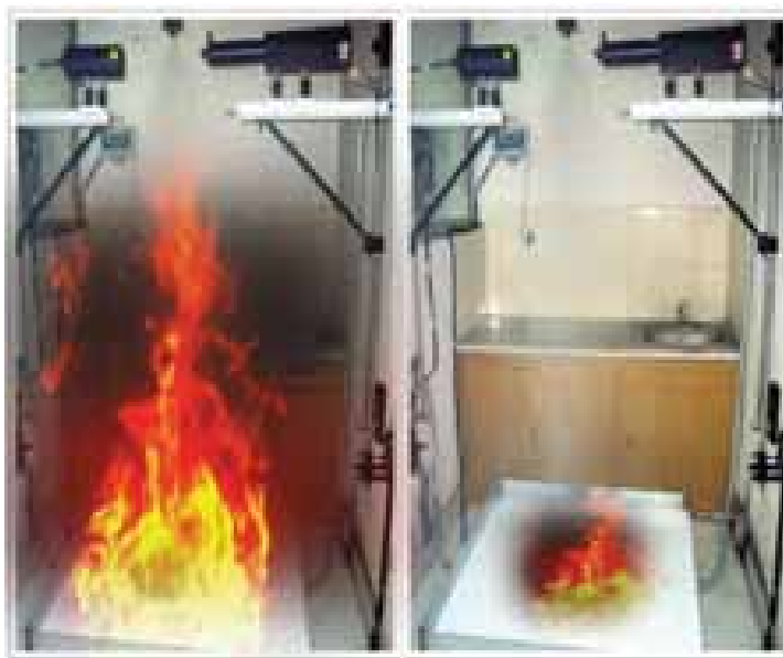
Fig.2: Experimental facility for development of low ODP (0.01 to 0.5) fire extinguishants Experiments Measurements:
