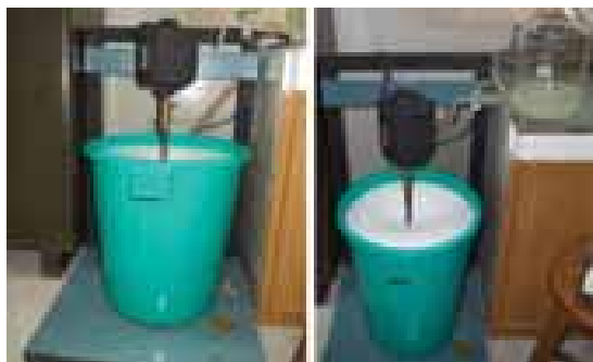
Fig.1: Set up for bench scale preparation of silica nanoparticles
