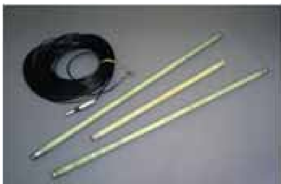
Fig.2: Borehole antenna probes with fibre optic cables
