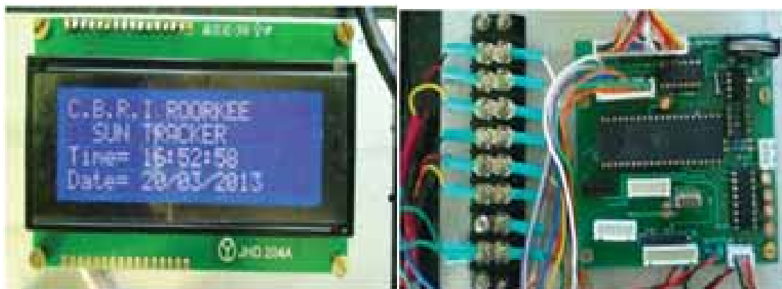
Fig.2: Solar Tracker - Micro Processor based electronic control
