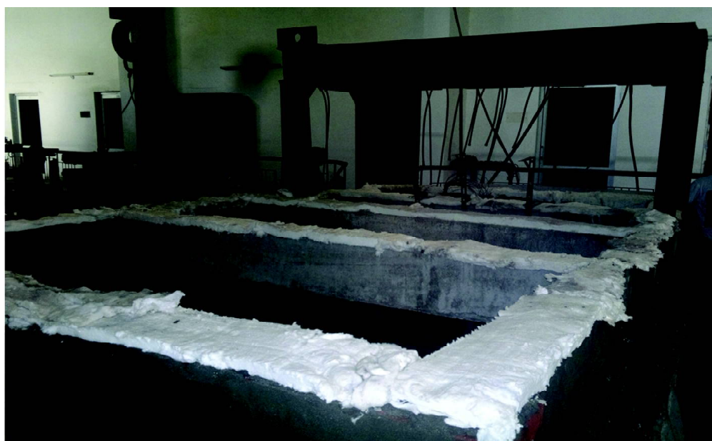
Fig.1: Test set up for fire resistance of beam
