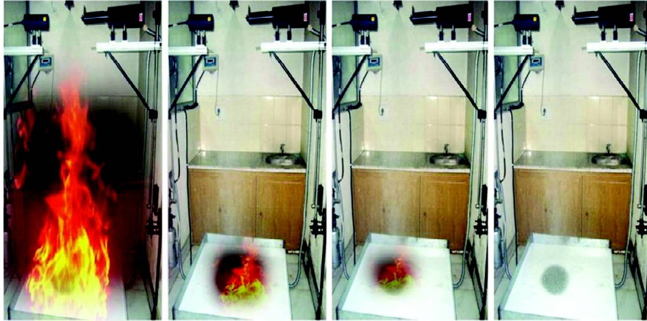
Fig. 2: Experiments with water-mist and other indigenously developed liquid extinguishants in the 18,000nm to 10,00,000nm size range for determining the effective sauter mean diameter for particle size distribution required for effective extinguishment.
