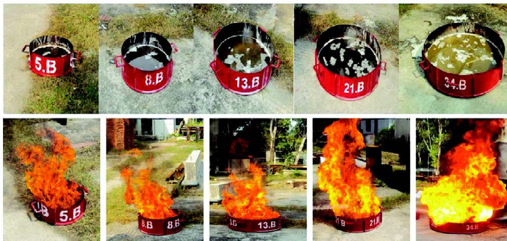
Fig.7: A new facility for water-mist fire extinguishers characterization of different size Class B Fires.
