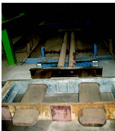
Fig.1. Wooden gang mould and Core withdraw Assembly
