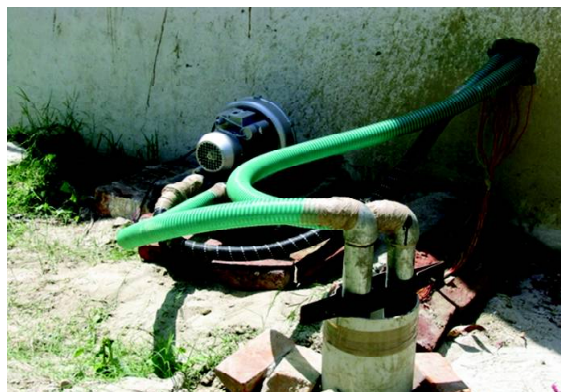
Experimental setup showing air-blower and U-shaped heat exchanger in bore-hole.
