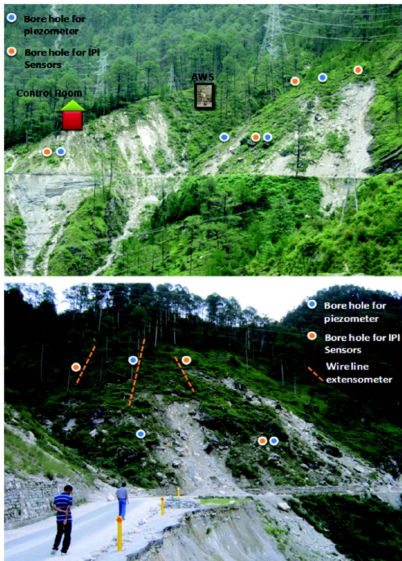
Scheme of field instrumentation at landslide site
