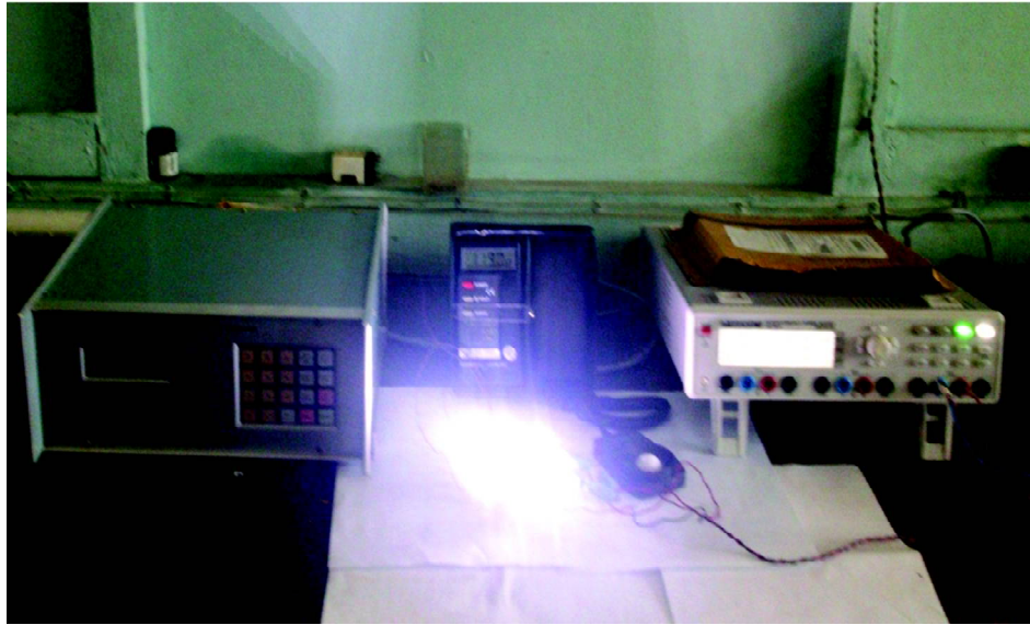
Fig.1: LED Bulb Electrical Characterization test setup
