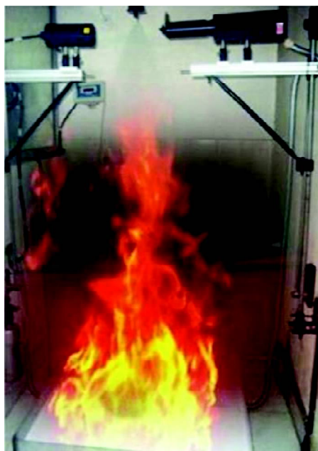
Fig.8: Characterization of newly developed zero (“0”) ODP Fire Extinguishant with fire suppression time brought down from 30s to 15s.
