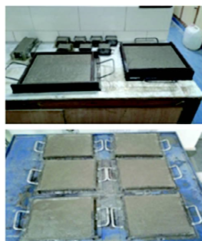
Casting of Vermiculite tiles and samples in Environmental Chamber
