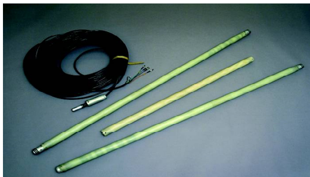
Fig 2: Borehole Antenna probes with fibre optic cables
