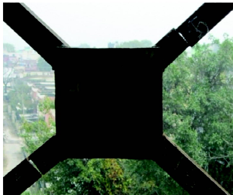
(a) Stiffness variation by cutting brace at 4 th floor
