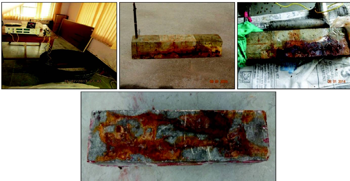
Fig.10 (a to g): Various phases of corrosion acceleration on beams
