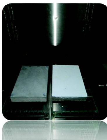
Casting of Vermiculite tiles and samples in Environmental Chamber
