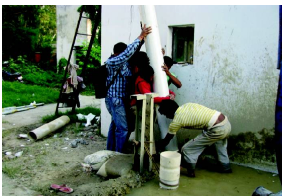
Experimental setup showing air-blower and U-shaped heat exchanger in bore-hole.
