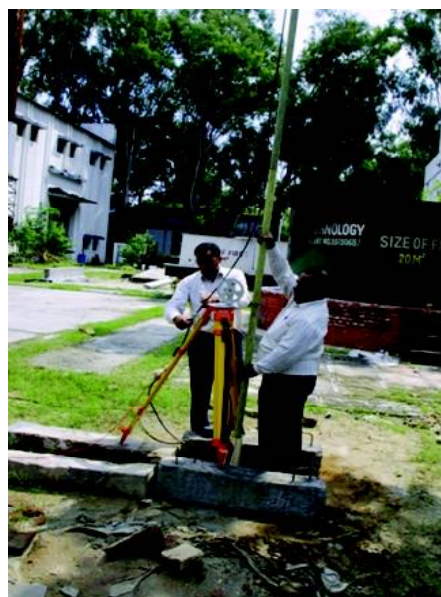
Assembly of Borehole Radar and its lowering in Borehole
