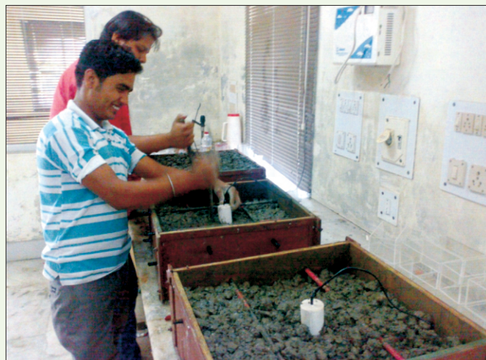
Fig. 2: Casting of RC specimen with galvanic anode
