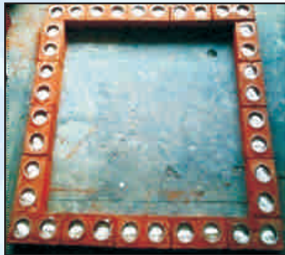
Fig 1: Experimental Set up of ordinary and PCM incorporated brick
