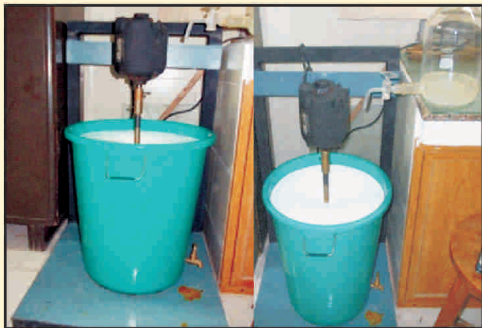
Fig.1: Set up for bench scale preparation of silica nanoparticles.
