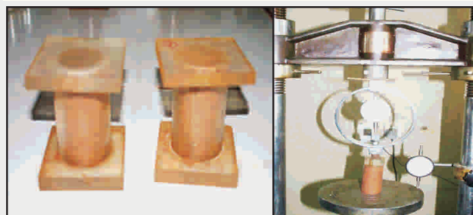
Fig. 1: Unconfined Compression Test
