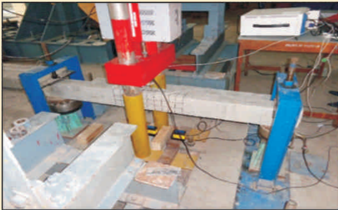
Fig. 1 (a): Support system to support beam and load cell
