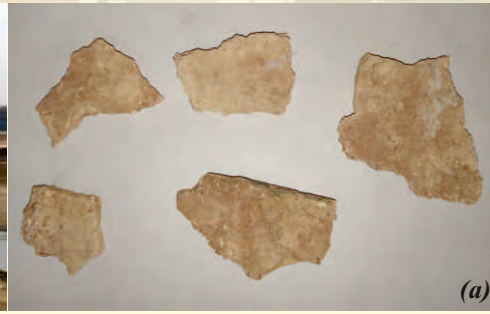
Fig. 2: (a) Mortar and (b) Brick Sample of Solani Aqueduct
