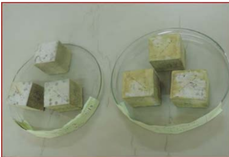
Fig.1: Bacterial and control specimens immersed in acid
