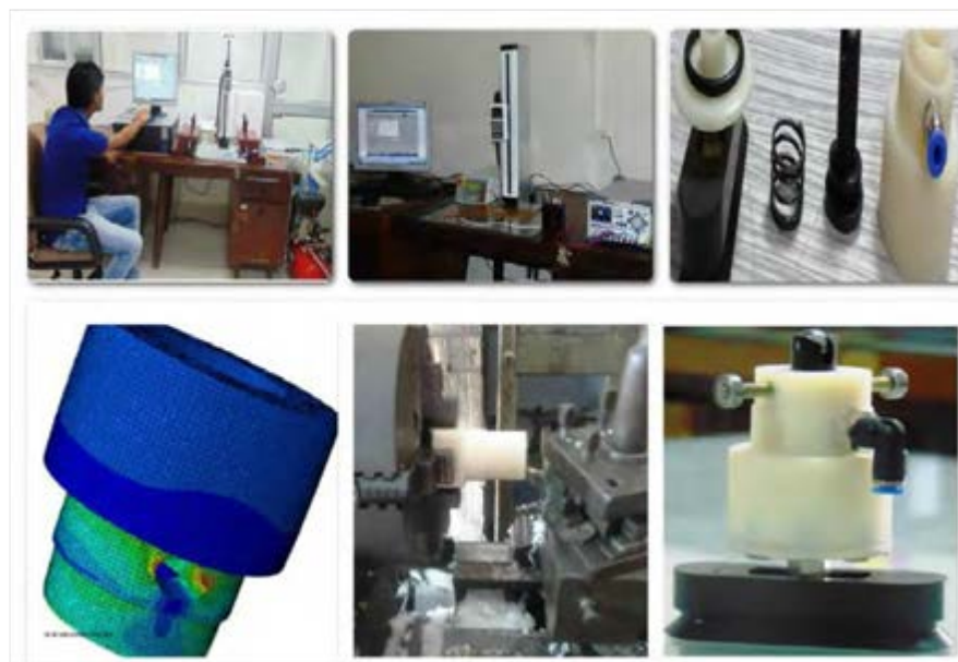
Fig. 1: Testing, design and development of adhesion mechanism for glass facade cleaning robot
