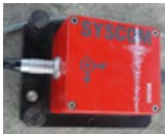
(b) Wired velocity sensor
