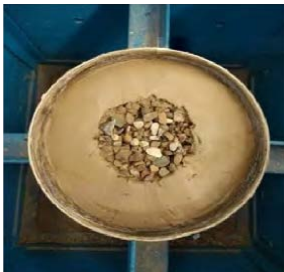
Fig. 1: View of stone column and unit cell
