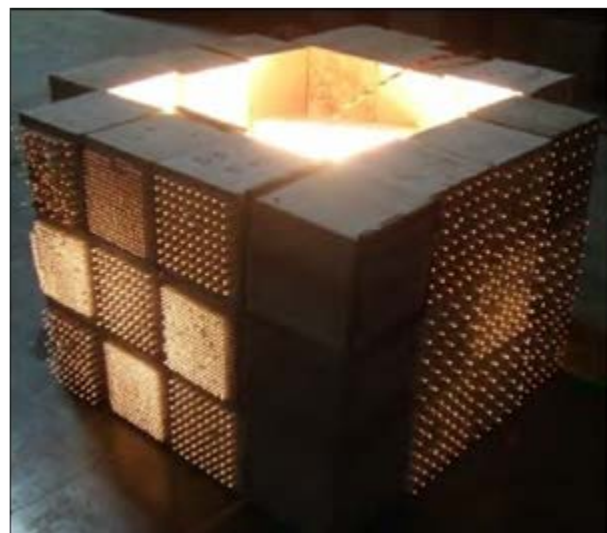
Fig. 4: View of translucent concrete
