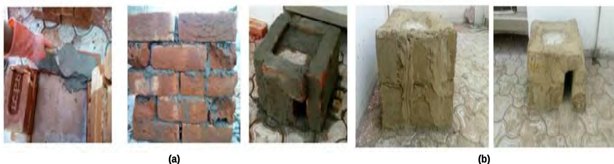
Fig. 7: Small scale model house (a) conventional using bricks and concrete (b) mud composite.
