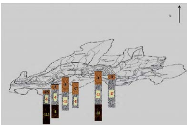
Fig. 2: Subsurface model of vs based on seismic refraction survey at left side of river at Srinagar
