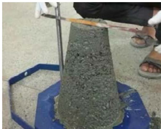
Fig. 3: Slump value - 0 mm.
