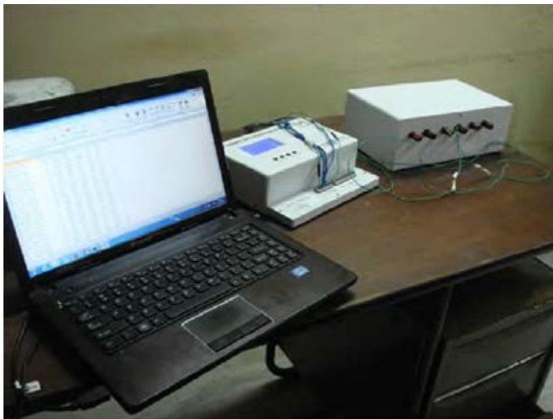
Fig. 4: CP monitoring system
