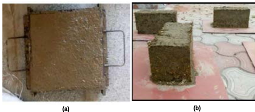
Fig. 6: Stabilized mud composites (a) mud phuska roof tile (b) wall blocks
