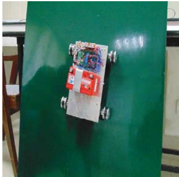
Fig. 1: Developed autonomous climbing machine
