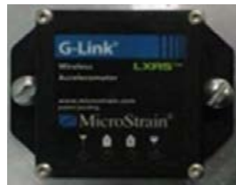
(e) Wireless accelerometer
