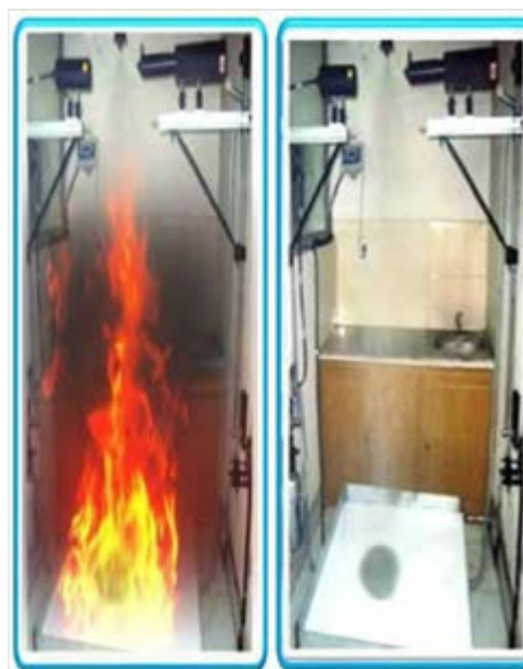
Fig. 1: Design guidelines-related field trial experiments on novel water-mist and/or low ODP extinguishant fire suppression system based on water-mist technology, carried out on a working space of 3m(l) x 2m(w) x 2.75m(h).
