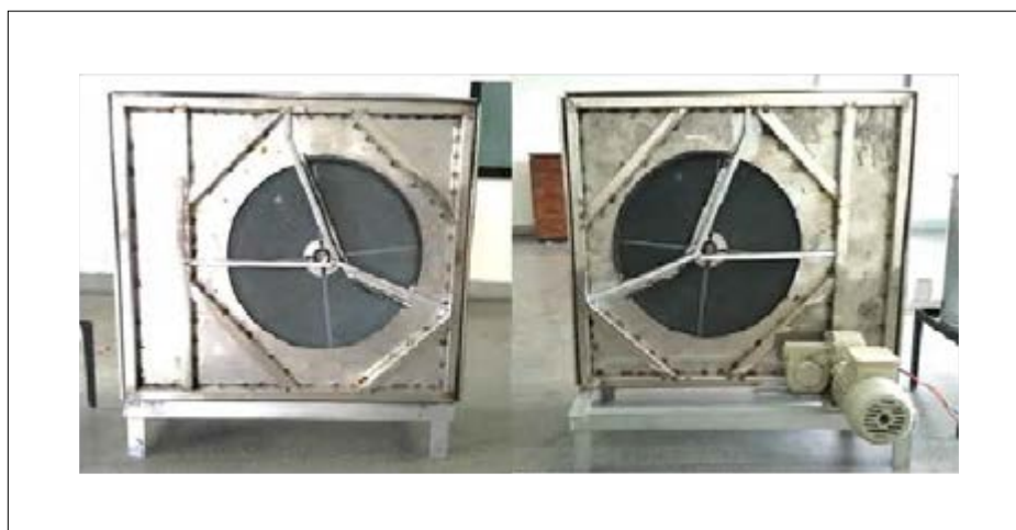
Fig. 7: Front and back view of fabricated desiccant wheel
