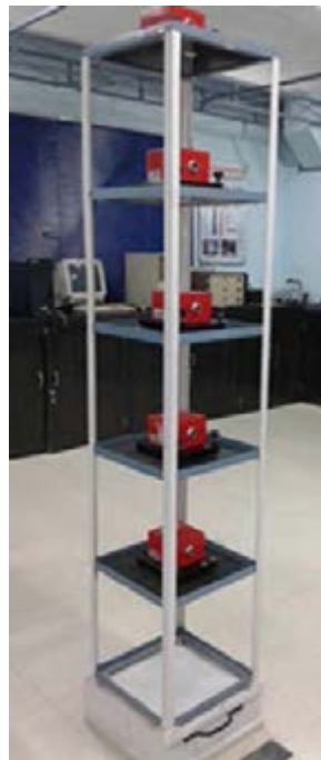
Fig. 3: Lab scale models of 5-storey steel frame, 8-storey steel building and 6-storey RC building
