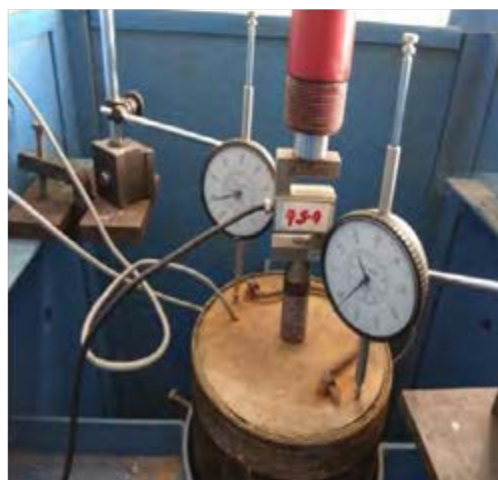
Fig. 4: View of complete load test set-up
