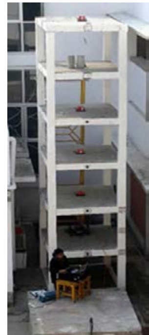
Fig. 3: Lab scale models of 5-storey steel frame, 8-storey steel building and 6-storey RC building
