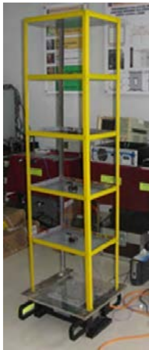
Fig. 3: Lab scale models of 5-storey steel frame, 8-storey steel building and 6-storey RC building
