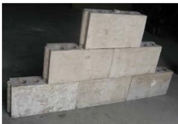
Fig. 3: Proposed wall from inter locking fluoro gypsum panels
