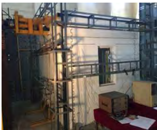
Fig. 2: Full-scale retrofitted confined masonry building subjected to lateral cyclic load
