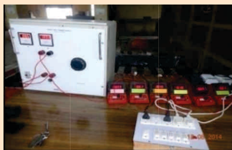
Fig. 2 (a to c): Scheme for corrosion acceleration and beams corrosion in progress
