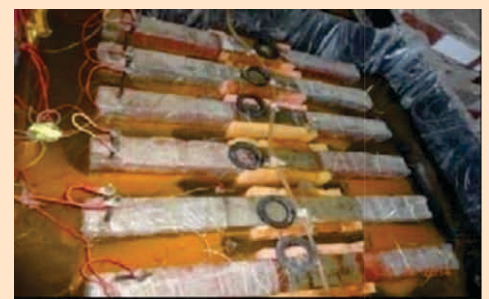
Fig. 2 (a to c): Scheme for corrosion acceleration and beams corrosion in progress
