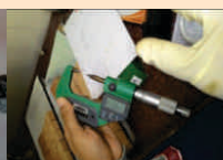
Fig. 5 (a to g): Gravimetric testing procedure (breaking of beams for rebars extraction, cleaning of rebars, weight/depth measurements & bars identifications)
