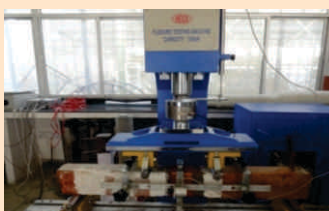
Fig. 6 (a to c): Structural test set up and beams testing in progress
