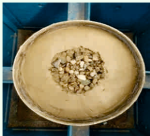
Fig. 1: View of stone column and unit cell
