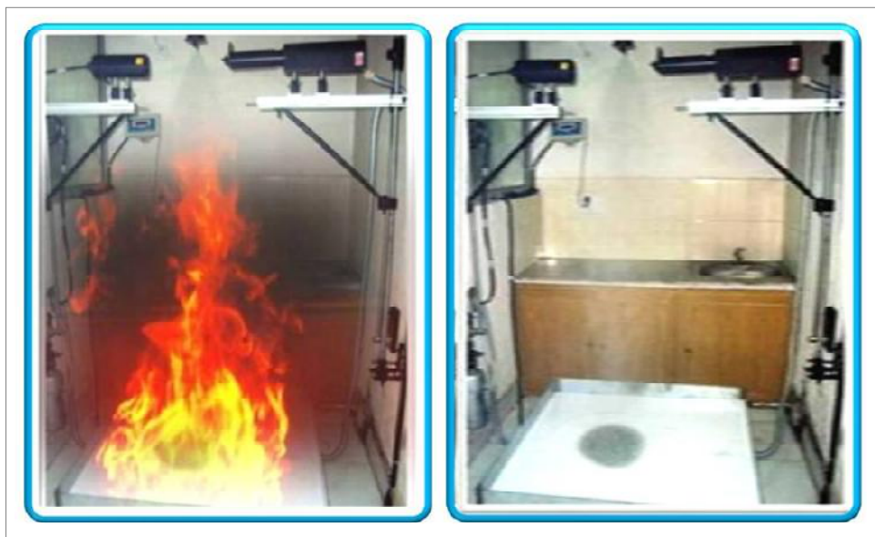
Fig 1: Revalidation with Field Trial of Novel Water-Mist and/or Low ODP Extinguishant Fire Suppression System based on Water-Mist Technology has been carried out on a Working Space of 3m(L)x2m(W)x2.75m(H)
