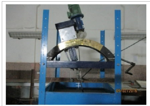
Fig 2: Experimental Setup Fabricated for Pull out Test at CSIR-CBRI, Roorkee
