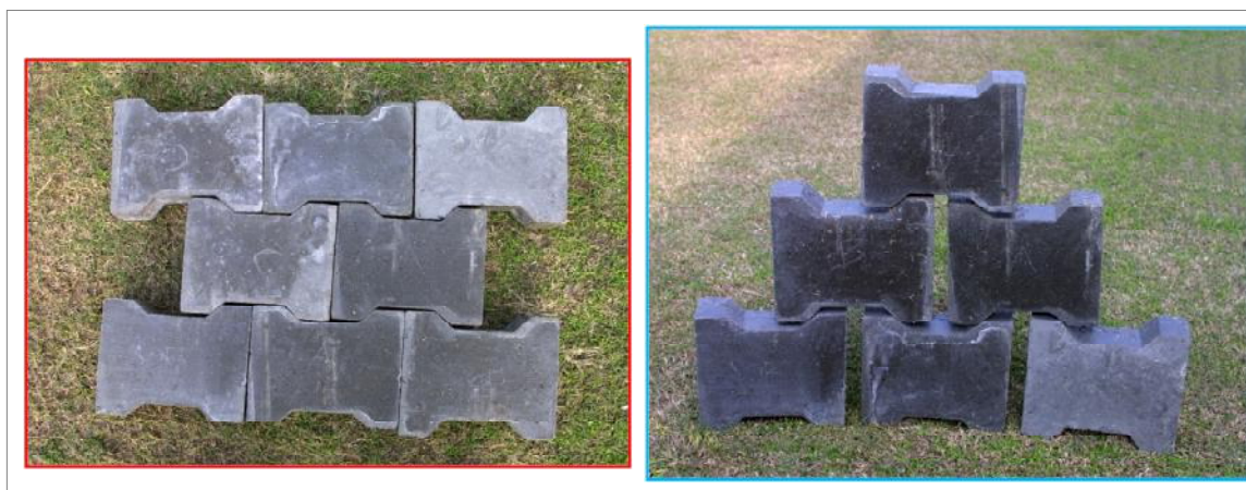
Fig 1: Two layered Interlocking Paving Prepared of Recycle Aggregate
