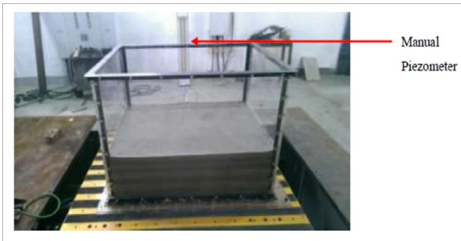
Fig 5: Test Setup for Liquefaction of Sand
