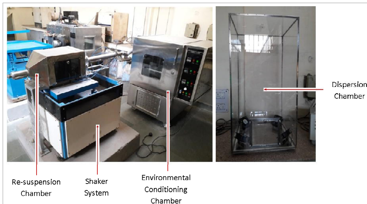
Fig 1: Experimental Set-up for Re-Suspension Studies
