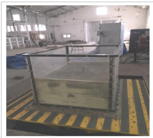
Fig 2: (a) Model Test Tank with the Sand Specimen
