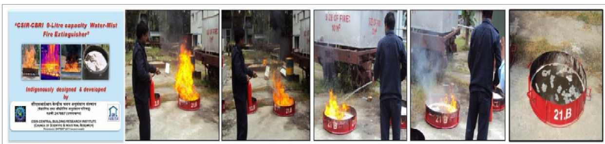
Fig 2: Field Trial of Class 21B Fires on Flammable Liquid Fires for Fire Extinguishing Performance Evaluation of the 9 litre Capacity Water-Mist Fire Extinguisher
