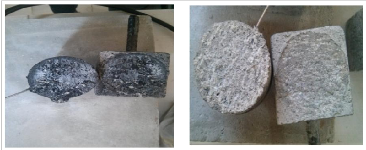
Fig 3: Overlay-Substrate Interface Failure
