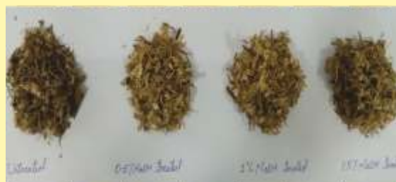
Fig. 2: Chemically treated and untreated fibres
