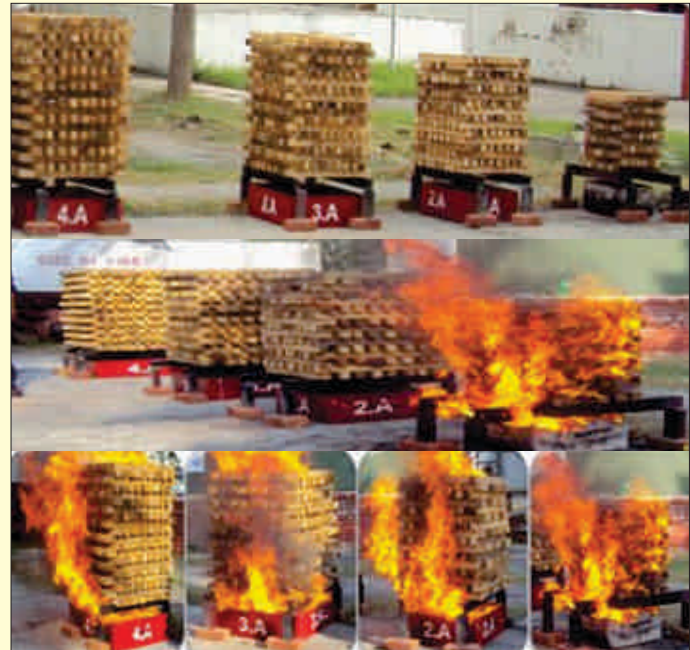
Fig. 1: New facility developed for optimization of compositions based on fire suppression efficacy for water mist system and comparative evaluation of on micro-size particles in discharge cluster as per IS:15683-2006 on Class A wooden-crib fires.
