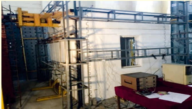
Fig. 2: Full-scale retrofitted confined masonry building subjected to lateral cyclic load
