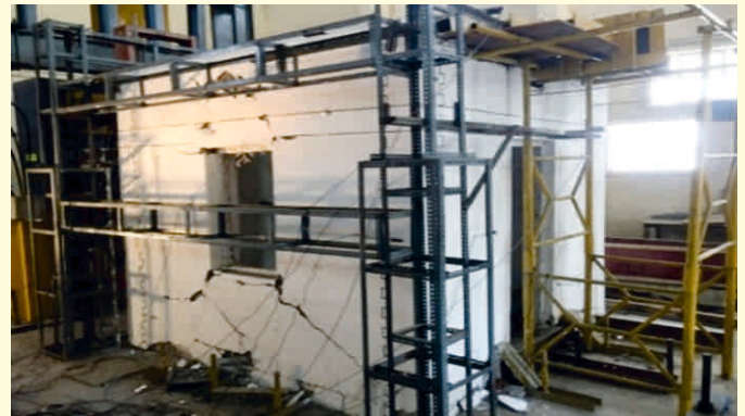
Fig. 3: Damage pattern for retrofitted confined masonry building subjected to lateral cyclic load
