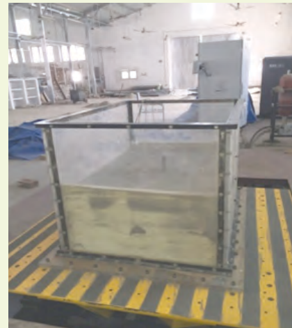
Fig. 2: (a) Model Test Tank with the Sand Specimen
