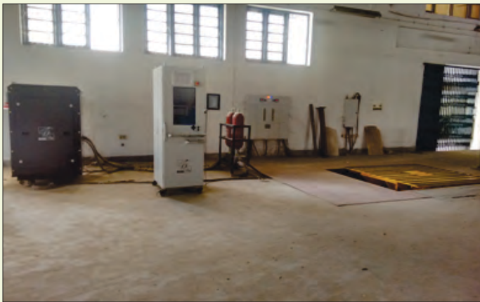
Fig. 1: Uni-Axial Shake Table & its Accessories
