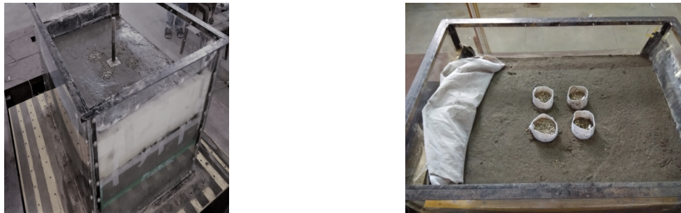
Fig. 1: Test Assembly for the Shake Table Test on Saturated Sand Reinforced with (a) Ordinary Stone Columns (b) Encased Stone Columns Area Replacement Ratio (2.6%)
