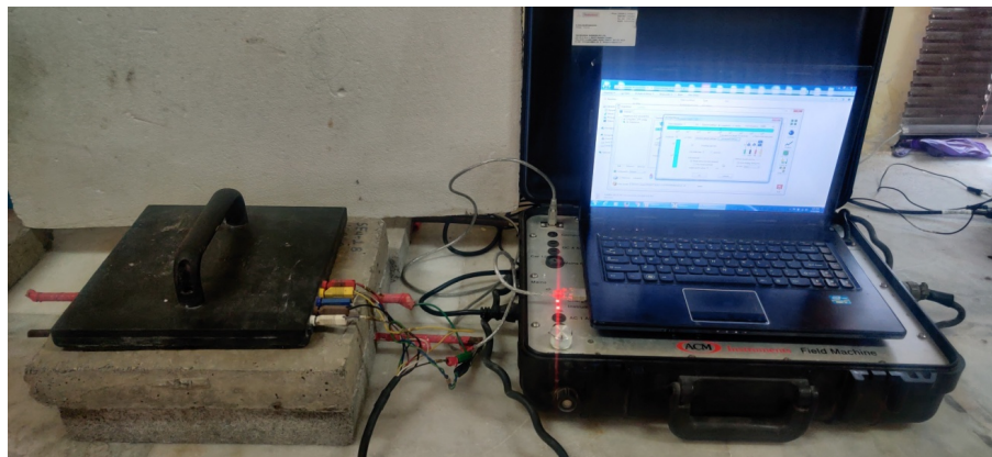
(a) The Setup for Testing of Corrosion in Laboratory
