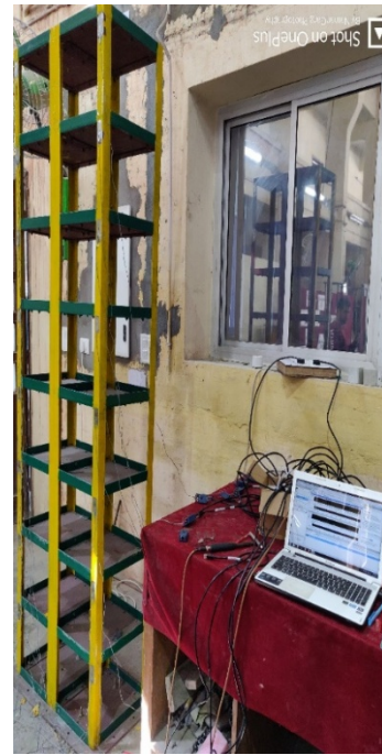
Fig. 3: : Instrumented 6-Storey 2-Bay Steel Structure
