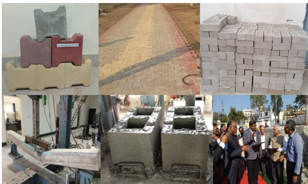
Fig. 1: Photographs of Building Components developed using C&D Wastes, Baggase Ash, RMC Sludge, Rice Husk Ash
