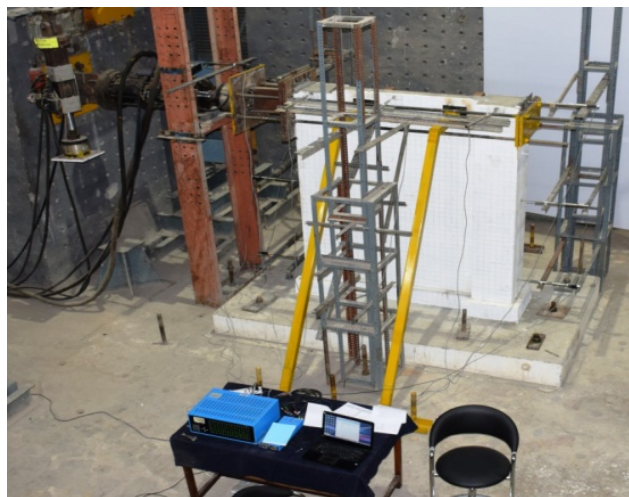
Fig. 1: Test Set-Up for Precast RC Walls
