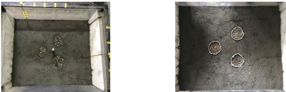
Fig. 2: Test Assembly for the Shake Table Test on Saturated Sand Reinforced with (a) Ordinary Stone Columns (b) Encased Stone Columns Area Replacement Ratio (5%)
