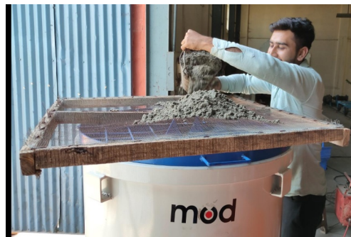
Fig. 3: Putting Sand & Cement Mixer in Mortar Spraying Unit
