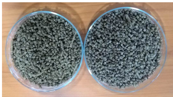
Fig. 2: Extruded Pellets of Thermoplastic Bamboo Composite
