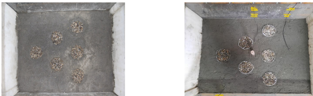
Fig. 3: Test Assembly for the Shake Table Test on Saturated Sand Reinforced with (a) Ordinary Stone Columns (b) Encased Stone Columns Area Replacement Ratio (9.6%)
