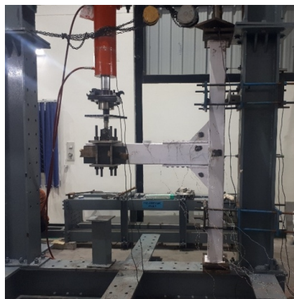
Fig. 1: General Configuration Experimental Test Setup Beam Column Joint
