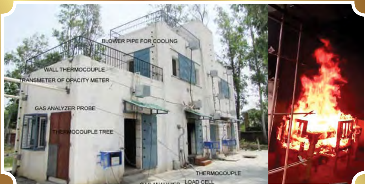
Full scale fire experimental facility for G+1 building
