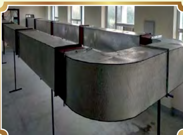
Test Bed Duct Facility for COVID-19 disinfection solutions
