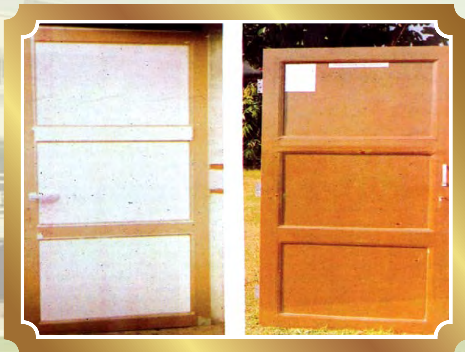
Aluminium and Mild Steel Door shutters exposed to flames
