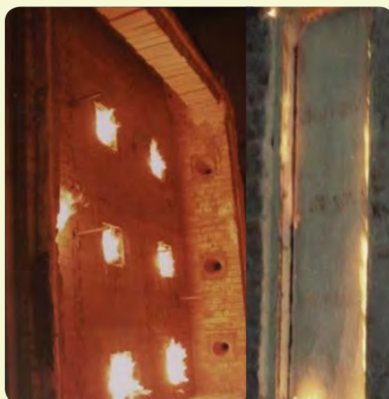
A fire door with a specific fire-resistance rating is used as part of a passive fire protection system to reduce the spread of fire from one compartment to other and to enable safe egress from a occupancy.
