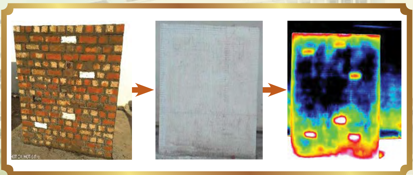
Defect detection in plastered Masonry wall using Thermal Imaging
