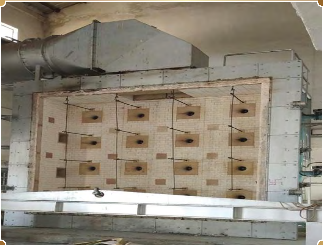
Vertical wall furnace for testing fire resistance of building elements
