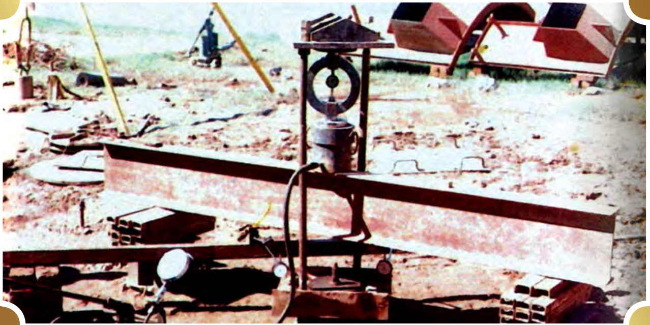
Test set up for single pile
