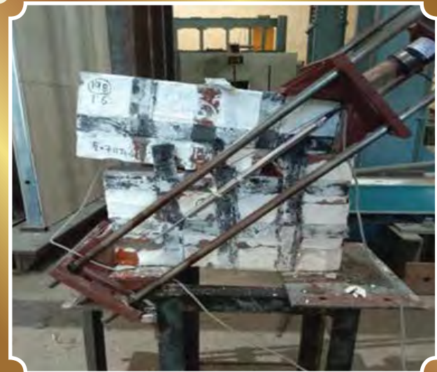
Modified Diagonal Compression Testing of FRP Strengthened Brick wall
