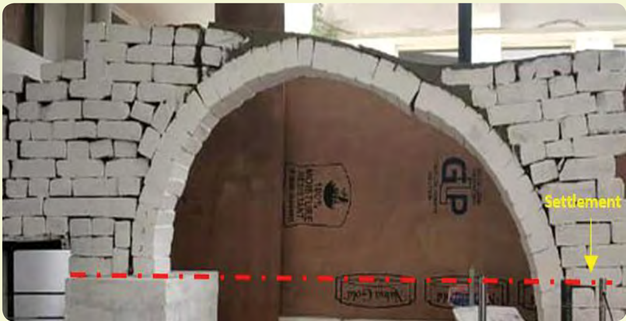
Masonry Arch under Support Settlement
