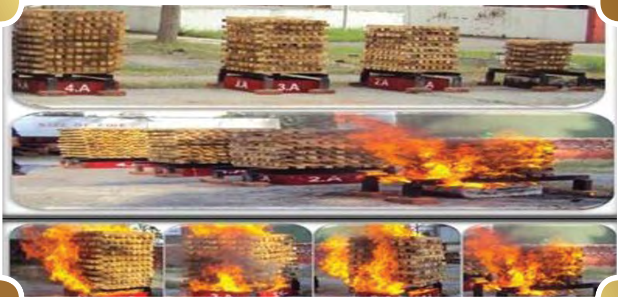
New facility developed for optimization of compositions as per IS: 15683-2006 on Class A wooden-crib fires
