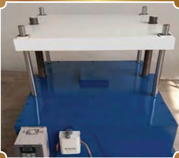
Development of controlled settlement mechanism
