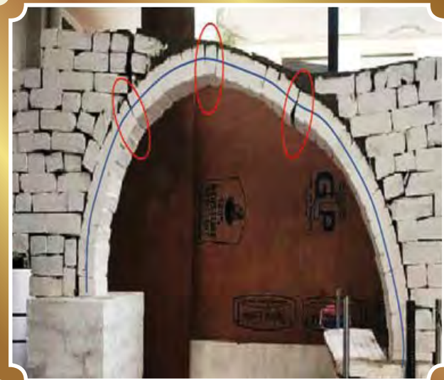
Monitoring of dry stack arch structure under settlement using FBG sensors
