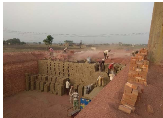
High draught Brick kiln with Zig-zag Setting as designed by CSIR-CBRI, Roorkee
