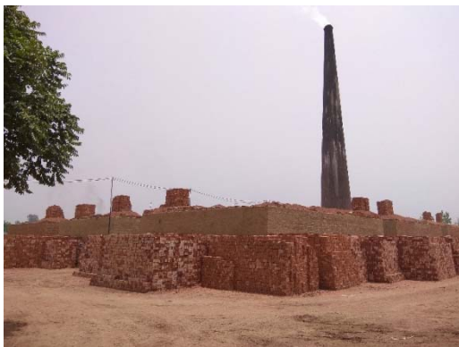
High draught Brick kiln with Zig-zag Setting as designed by CSIR-CBRI, Roorkee
