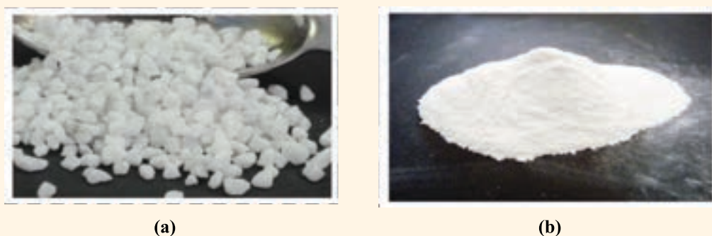
Fig. 1 Processed Marble Waste(a)Aggregate and (b) Powder Waste
