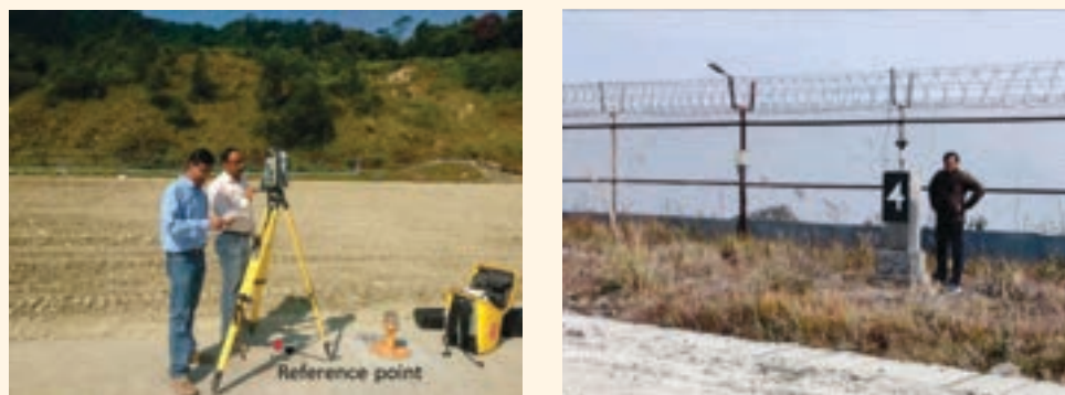
Fig.5. Monitoring of RE wall from runway level
