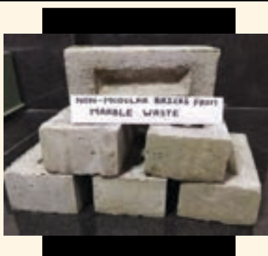
Fig. 4. Developed non-modular bricks using marble waste
