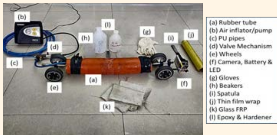
Fig. 4. The integrated mechanized retrofitting system.
