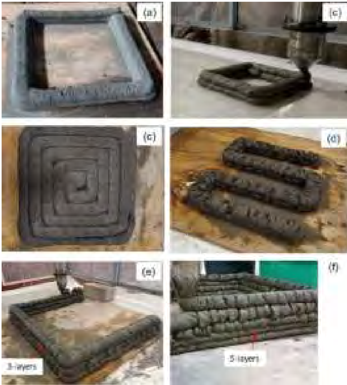
Fig. 4 (a)-(e) Experimental concrete printing trials using various mix design at laboratory level.
