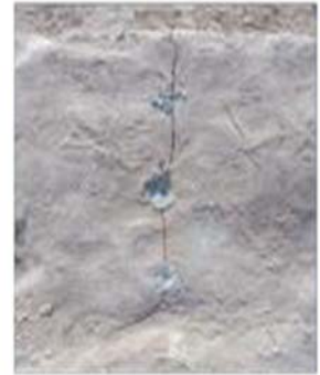
Cracking pattern of CBRI silent cracking mortar
