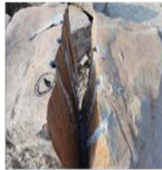
Cracking pattern of CBRI formulation cracked after 15h
