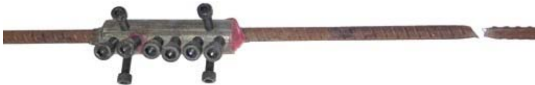
Rebar with Coupler: Failure away from Coupled region.
