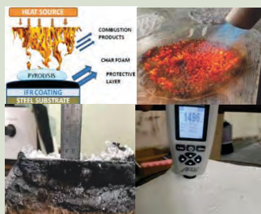
Fire retardant intumescent coating for steel and GI duct applications
