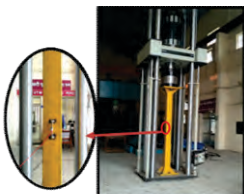
300T UTM and SHM of using FBG, VWSG etc.
