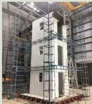
Full Scale Testing of 3D Volumetric Construction
